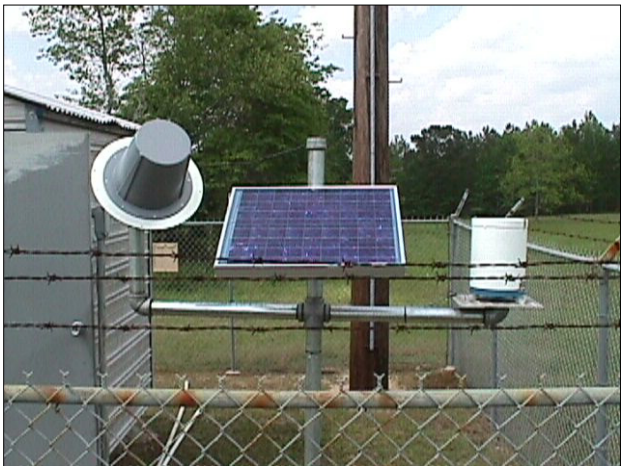
Figure 5-2 Typical Field Installation of Precipitation Gage
