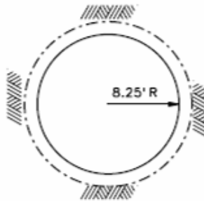
TYPICAL SECTION CIRCULAR CONCRETE-LINED TUNNEL TO STATION 11+51
